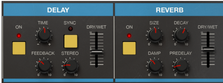
The two extra effects added by Arturia to the Jun-6 V, present in the Advanced Panel: Delay and Reverb.
