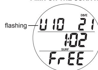
VIOLATION AFTER 1 MIN ON THE SURFACE
