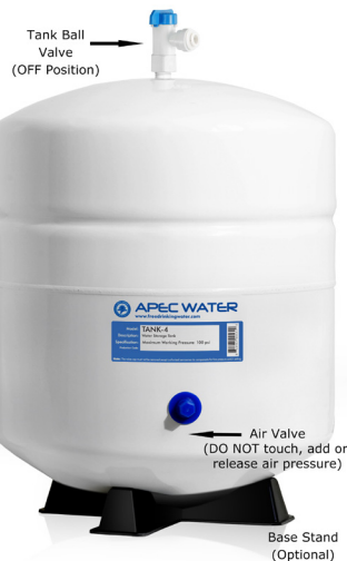
Standard 4-gallon Tank Diagram:
