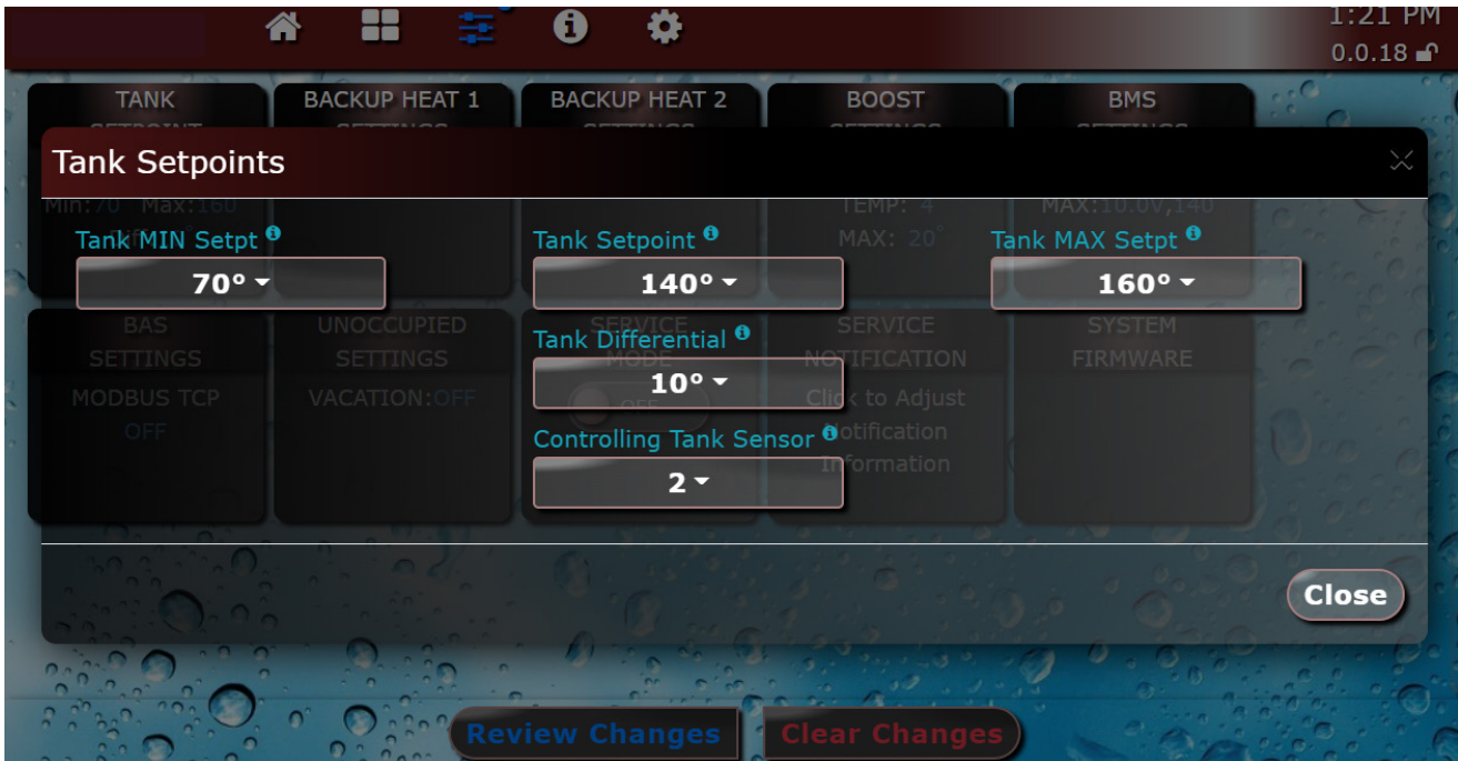
Figure 1-3 Tank Setpoints HW Screen
