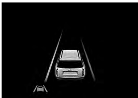
Lane Departure Warning (right)
