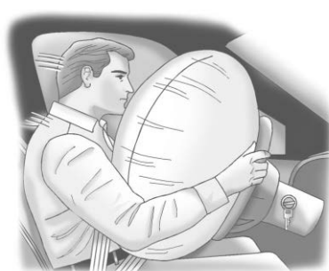
The driver frontal airbag is in the center of the steering wheel.
