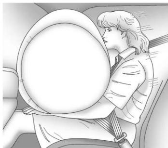
The front outboard passenger frontal airbag is in the passenger side instrument panel.
