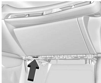
Interior Power Outlet
