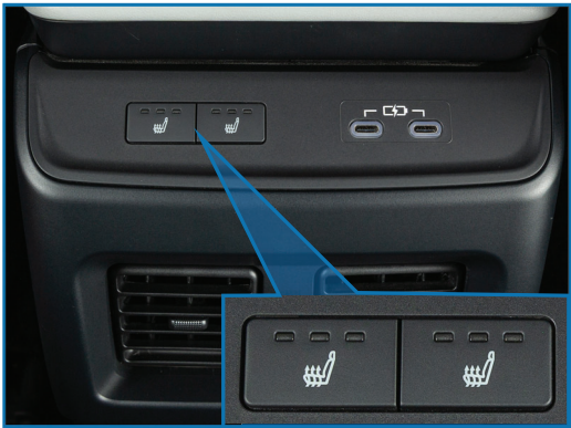
Rear Heated Seat Switches
