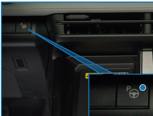
Advanced Park Main Switch
