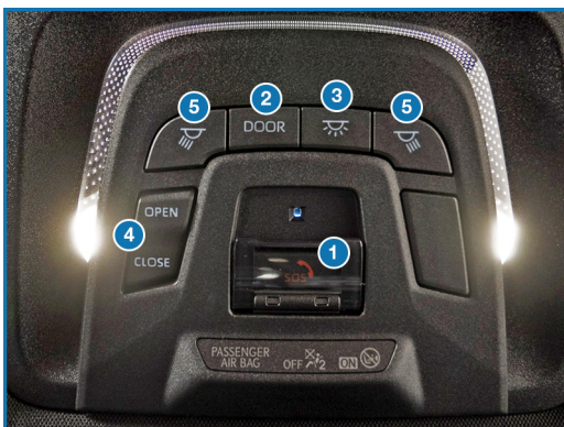
Overhead Console Switches
