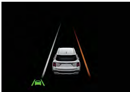
Lane Departure Warning (right)
