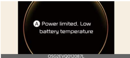
A: Power limited. Low battery temperature
