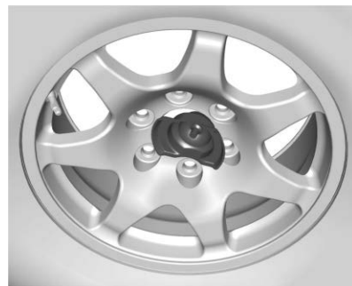
All Other Models Incorrectly Stored, Retainer Off-Center
