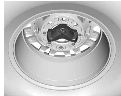
AT4X Model Correctly Stored, Retainer Centered
