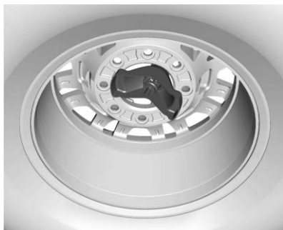
AT4X Model Incorrectly Stored, Retainer Off-Center
