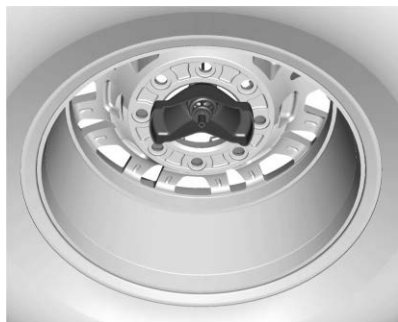
ZR2 Model Correctly Stored, Retainer Centered
