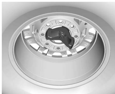
ZR2 Model Incorrectly Stored, Retainer Off-Center
