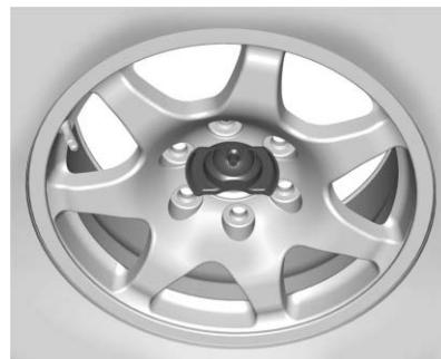
All Other Models Correctly Stored, Retainer Centered
