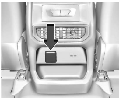
Rear of Center Console Power Outlet
