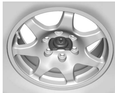
All Other Models Correctly Stored, Retainer Centered
