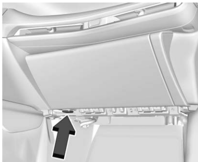
Interior Power Outlet
