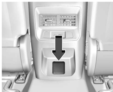
Rear of the Center Console Outlet
