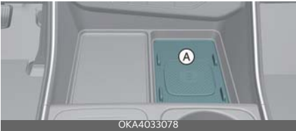
A: Charging pad
