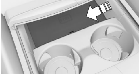
Tray with thermoelectric cup holder:
