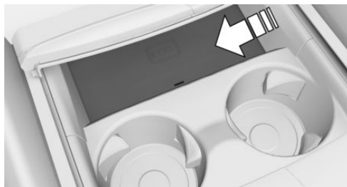
Tray with thermoelectric cup holder:
