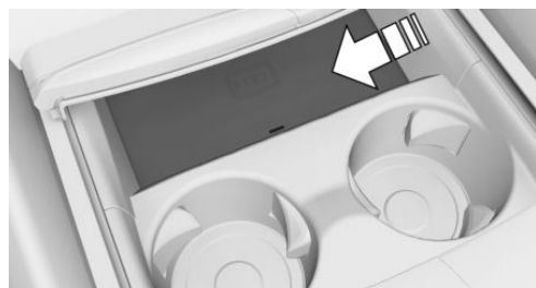
Tray with thermoelectric cup holder:
