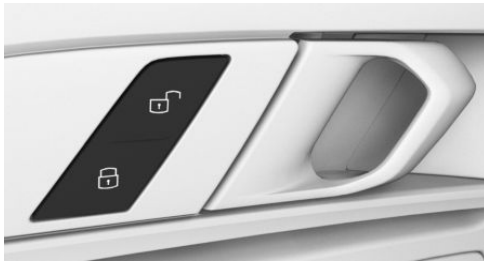
Buttons for the central locking system.
