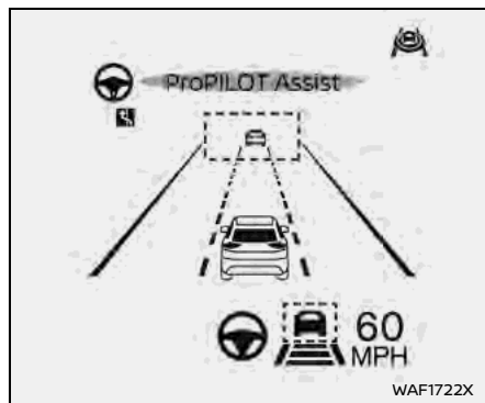
System set display — a vehicle detected ahead (for ProPILOT Assist 2.1)
