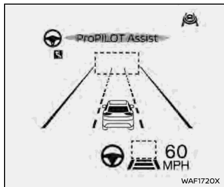
System set display — no vehicle detected ahead (for ProPILOT Assist 2.1)
