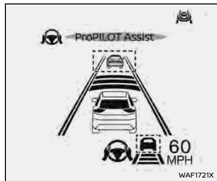
System set display — a vehicle detected ahead (for ProPILOT Assist, ProPILOT Assist 1.1)*
