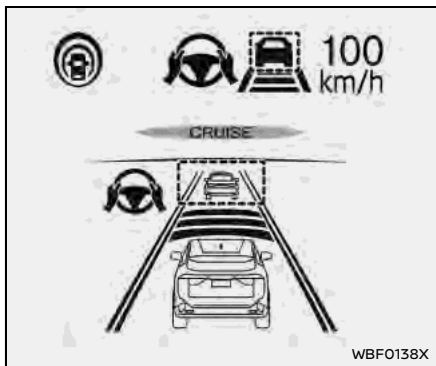
System set display — a vehicle detected ahead (for ProPILOT Assist with Navi-link)
