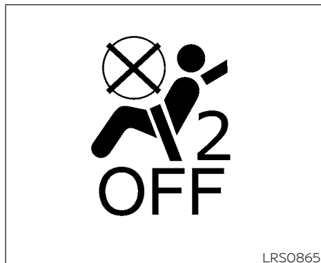
Front passenger air bag and status light
