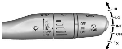
Windshield Wiper without Rainsense (INT Shown)
