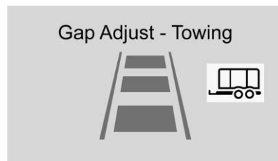
Far Gap Setting with Trailer
