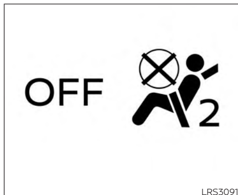
Front passenger air bag and status light
