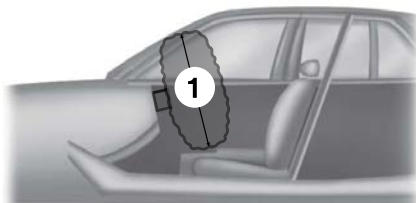
Figure 2 - Side View of the Driver Airbag at Full Inflation
