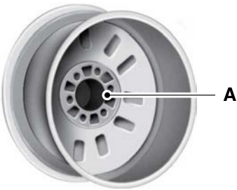
A Hub pilot bore.
