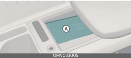
A: Charging pad
