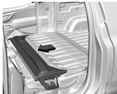
Midgate Lowered with Crossbar Attached
