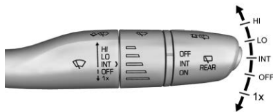
Windshield Wiper without Rainsense (INT Shown)
