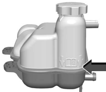
6.2L V8 Engine Coolant Surge Tank
