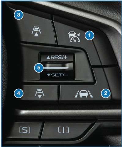
Adaptive Cruise Control Switches
