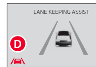
When the front-view camera does not detect the lane traveled in, the lanes are gray.
