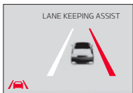
When the front-view camera detects the vehicle moving outside of the lane it is traveled in, the vehicle crossing lane will blink, either on the left or right lane (as shown in both images above)
