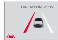
When the front-view camera detects the vehicle moving outside of the lane it is traveled in, the vehicle crossing lane will blink, either on the left or right lane (as shown in both images above)
