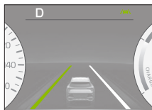
When LKA detects the vehicle moving outside of the lane being traveled in, a yellow lane marker will illuminate either on the left or right lane (shown in both images above)
