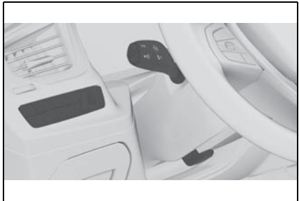
The light switch element is located next to the steering wheel.
