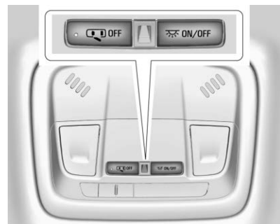
Dome Lamp Controls
