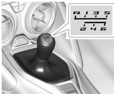
Shift Pattern – L4 and V6 Engines
