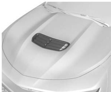
Hood Air Extractor
