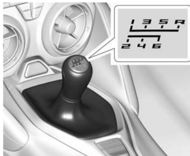
Shift Pattern – V8 Engine
