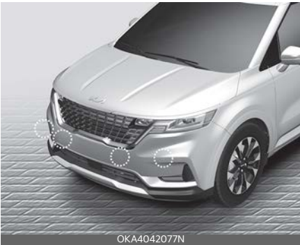
Front corner ultrasonic sensors
