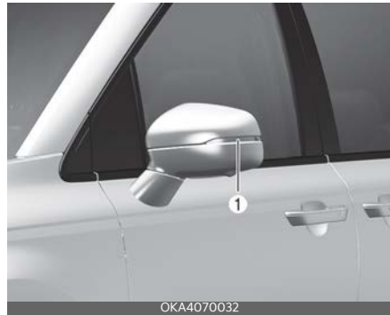
Light bulb position (Side)
