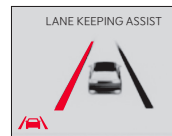
When the front-view camera detects the vehicle moving outside of the lane it is traveling in, a vehicle crossing lane indicator will blink, either on the left or right lane (as shown in both images above)
