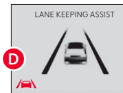
When the front-view camera does not detect the lane traveling in, the lanes are not illuminated gray
