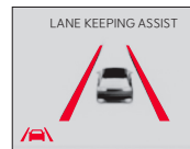
When the front-view camera detects the lane traveling in, both lanes are illuminated gray
