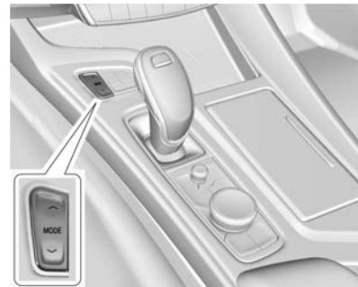
Driver Mode Control Switch for Automatic Transmission
