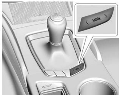
Driver Mode Control Switch for Manual Transmission
