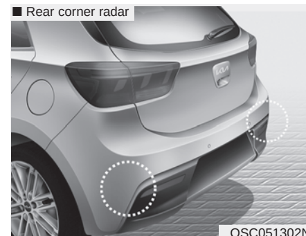
[A]: Rear Cross-Traffic Collision Warning operating range
