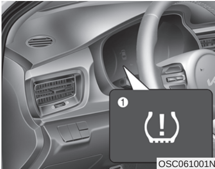
(1) Low tire pressure telltale/ TPMS malfunction indicator
