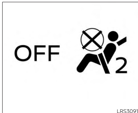
Front passenger air bag and status light
