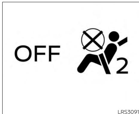
Front passenger air bag and status light
