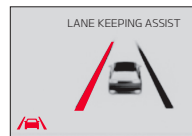
When the front-view camera detects the vehicle moving outside of the lane it is traveling in, a vehicle crossing lane indicator will blink, either on the left or right lane (as shown in both images above)
