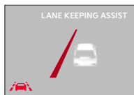
When the front-view camera detects the vehicle moving outside of the lane traveled in, a vehicle crossing lane indicator will blink, either on the left or right lane (as shown in both images above)
