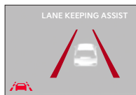
When the front-view camera detects the lane traveled in, both lanes are illuminated
