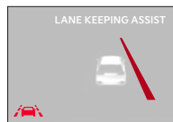
When the front-view camera detects the vehicle moving outside of the lane traveled in, a vehicle crossing lane indicator will blink, either on the left or right lane (as shown in both images above)
