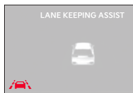
When the front-view camera does not detect the lane traveled in, the lanes are not illuminated
