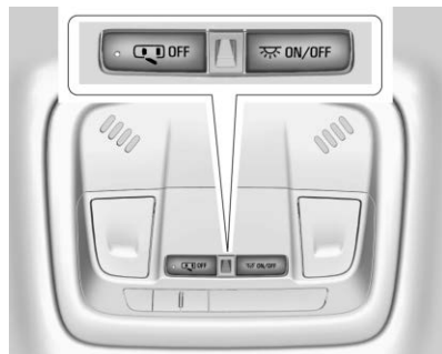
Dome Lamp Controls
