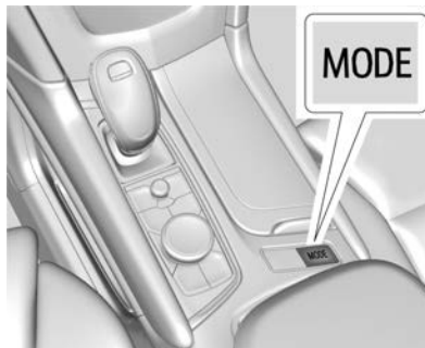
Driver Mode Control Switch
