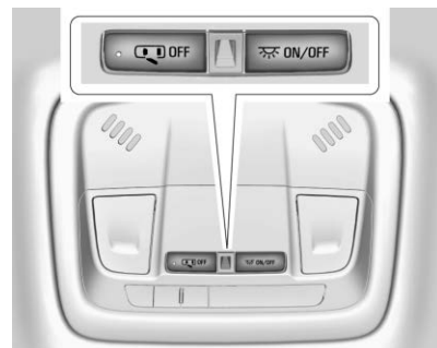
Dome Lamp Controls
