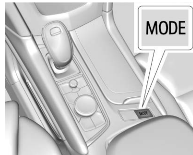
Driver Mode Control Switch
